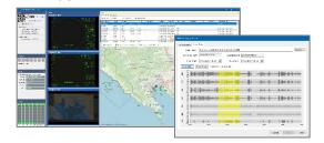
The AMI Marine Replay software is a unique tool that offers features like 'Audio Scan' and 'Jump to Incident.' These functions allow engineers, ship's crew, accident investigators, and even crew trainers to easily review data in an intuitive manner.
